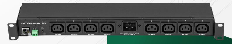
Each of eight outputs can be independently controlled from the web interface (switched on / off or power-cycled). To switch the outputs on in a sequence (after a power-up or when power is restored), a power-up delay interval can be configured for each output individually.
